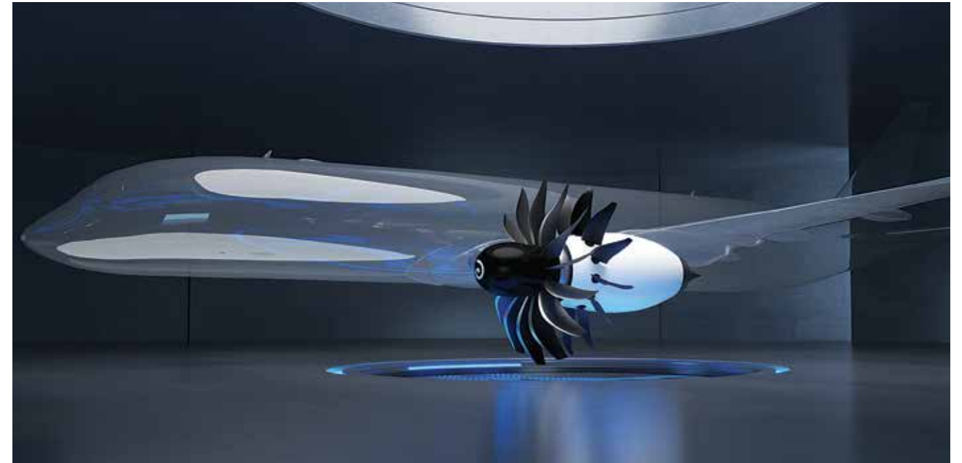
Through the RISE technology demonstration programme, CFM is advancing the development of its revolutionary Open Fan architecture, targeting up to 20 per cent greater fuel efficiency compared with today's most advanced engines
