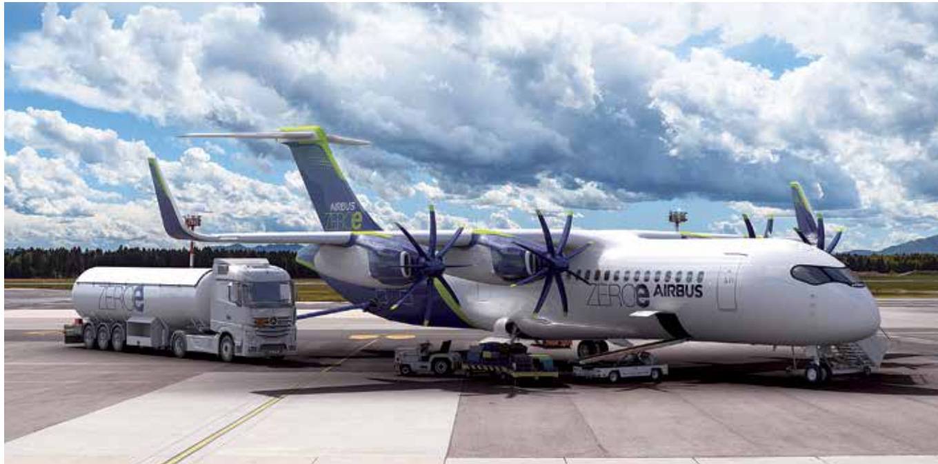
A mock-up image created to show what Airbus' fully electric, hydrogen-powered ZEROe aircraft will look like, and how it could be operated at an airport. It features four engines each powered by their own fuel cell stack.
