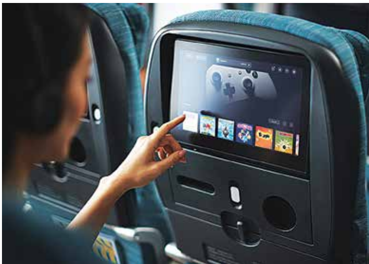
Smart Seat Display Unit has a high resolution capacitive touch screen, supporting touch gestures and an ability to play all formats of audio/video
