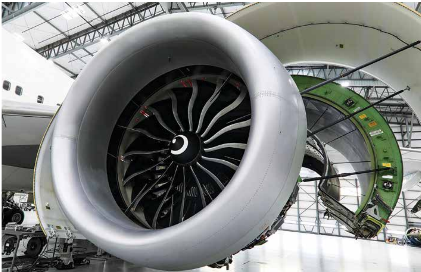
GE9X holds a Guinness World Record and is known as the most powerful commercial aircraft jet engine. Due to its advanced suite of technologies, the GE9X will deliver up to 10 per cent greater fuel efficiency.
