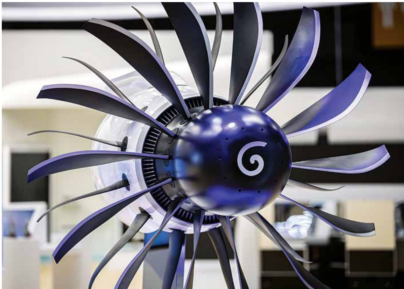
The CFM RISE (Revolutionary Innovation for Sustainable Engines) programme will be compatible with 100 per cent sustainable aviation fuel (SAF), capable of hybrid-electric operation, and possibly permit running on hydrogen
