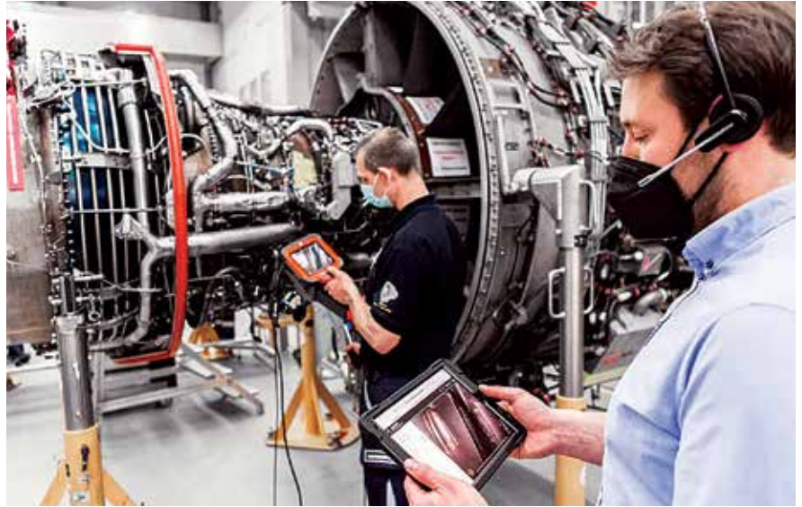
5G-assisted virtual borescopes performed on an engine in an overhaul shop
